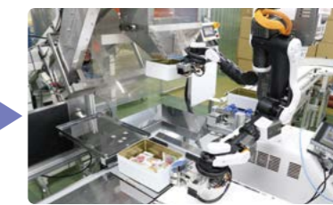
Based on the total weight, check the content amount and number of servings of crackers in the container. Forward to the next process only those that have successfully passed this phase.
