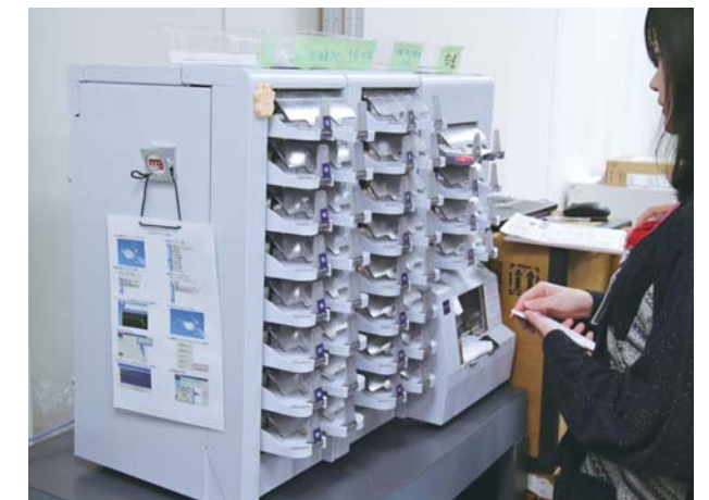
Using ballot-sorting machine to confirm that all name patterns are sorted correctly
