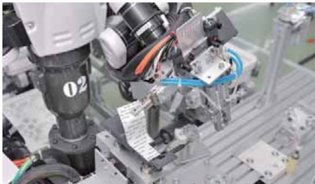
NEXTAGE robot stripping double-sided tape release paper
